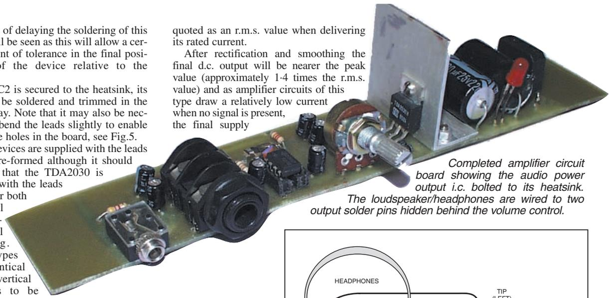
Completed amplifier circuit board showing the audio power output i.c. bolted to its heatsink. The loudspeaker/headphones are wired to two output solder pins hidden behind the volume control.
