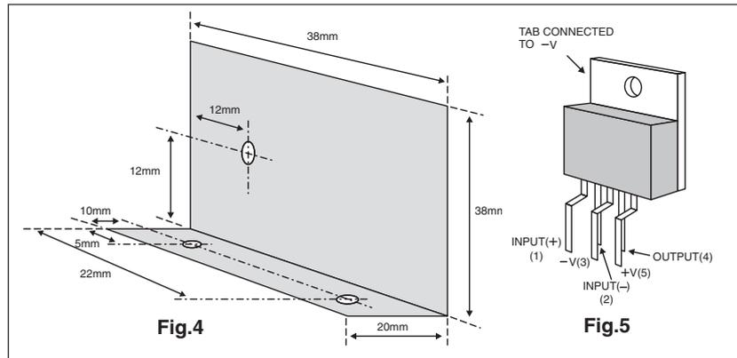
Fig.4 (top right). Heatsink dimensions and bending details.
